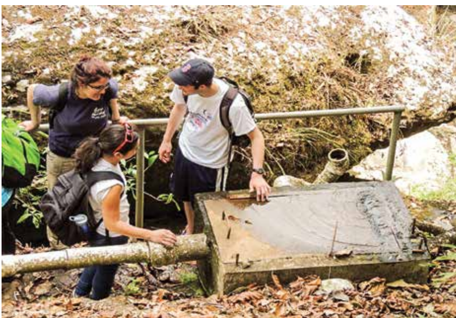
Samples and measurements are being taken at the combination box at the upstream end of the Cañazas water supply system.
